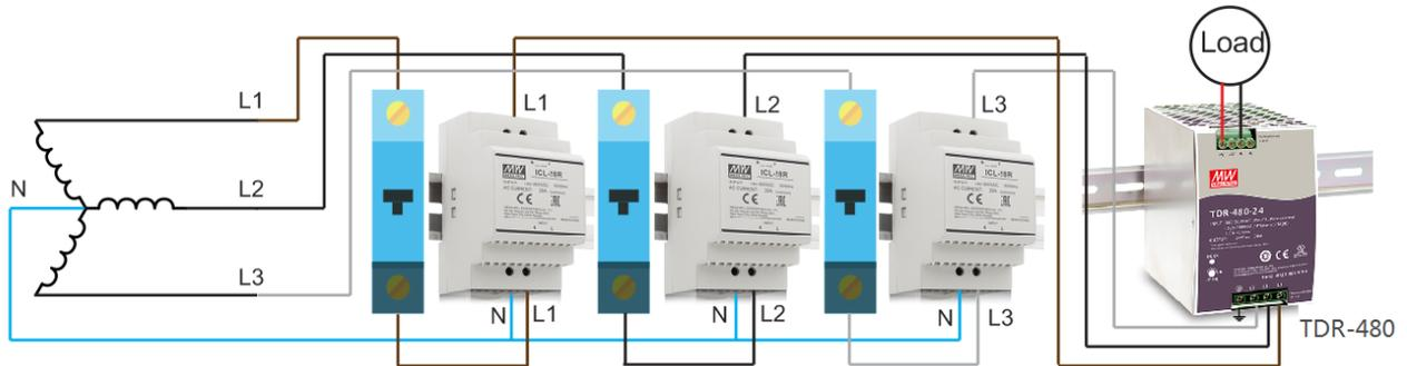
The power grid without the neutral line: It should be noted that the voltage between each live wire must not exceed 264VAC.
